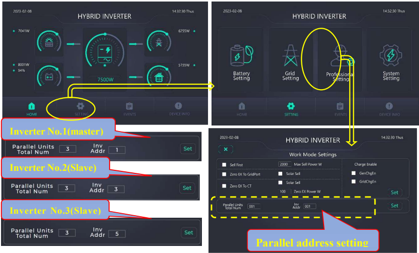
Figure 4.4 Enter the parameter setting diagram of the parallel machine and the address setting of the three machines
