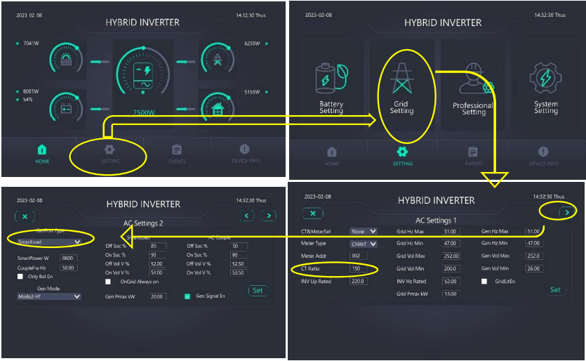
Figure 3.17 Intelligent Load and CT Ratio Setting Path
